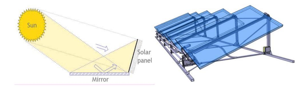
"Heat Mirror", located between the solar panels, scatter over the surface of the facade reflects electromagnetic waves. Mirrors are made of tempered glass shock hydrophobic self-cleaning surface and infrared heating - a system of anti-icing and snow melting in winter.
