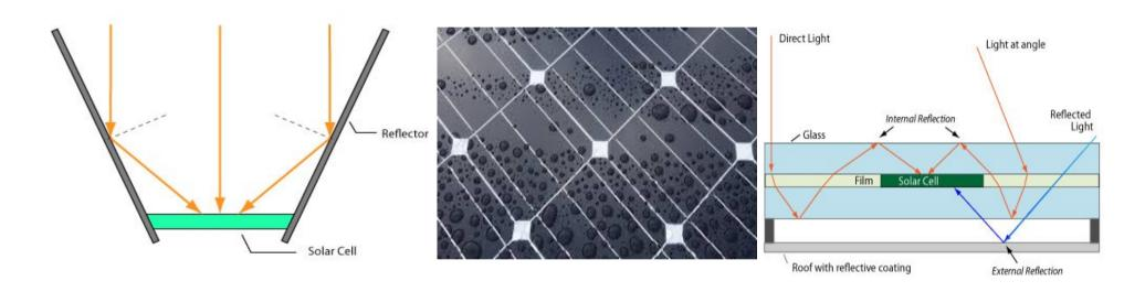
Over time, the working surface of the solar panels collects dust, which is able to significantly reduce the amount of electricity generated by batteries, efficiency panels may fall by 8-12 percent. In this regard, the surface self-cleaning panels processed surface - nanoscale hydrofob transparent film based on TiO2 (titanium dioxide). Nanocoatings protects the Station from static electricity, prevents icing process at low temperatures.
