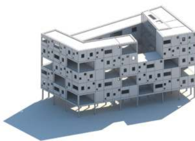
Pre fabricated panels
