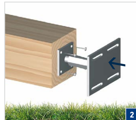
Connect the post anchor to the wood beam.
