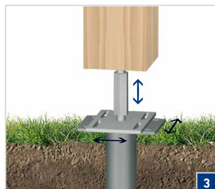
Place the post anchor (with post) onto the flange plate and align it.
