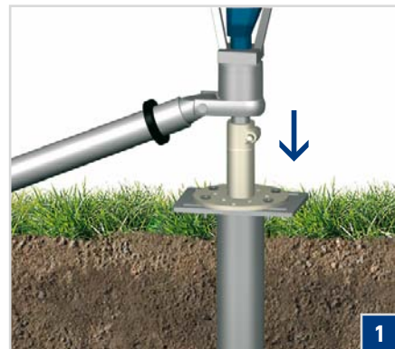
Drive the ground screw vertically into the earth.
