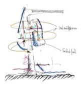
The architectural studio heri&salli from Vienna was assigned by the Vienna Technical Museum the development of a solar updraft tower for Vienna's urban space. In a solar updraft tower the air is warmed by the sun by means of a horizontal floor convector and rises due to the natural thermic convection in a "chimney". Several turbines create electrical energy by means of this airflow.
