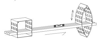
**STEP 6:** Once you have finalized the correct position, take out the bars and fix the second support to the wall (see step 3 and 4)
