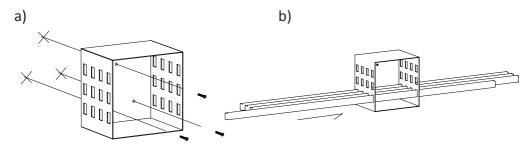
**STEP 5:** INSTALL THE SECOND SUPPORT. Slide the first set of bars into the second support. The level will help you to find the correct alignment
