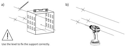
STEP 4: a) Screw the support to the wall b) Insert the first set of bars into the first support
