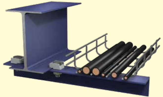
Cantilevered angle support for running cable tray
