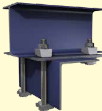
Angle section below an I-Section at 90 degrees
