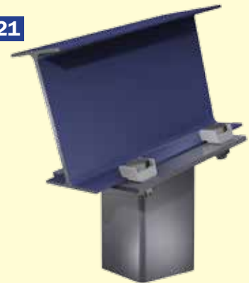
Column end plate to sloping I-Section
