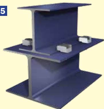
Drilled I-Section running parallel to another I-Section
