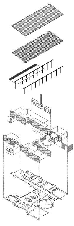
A standing-seam metal roof rests on top of a series of laminated wood beams.
