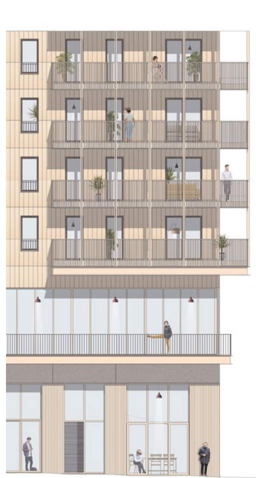
Facade of the E2B2 coliving building, with shared spaces on the 2nd floor, terracotta cladding
