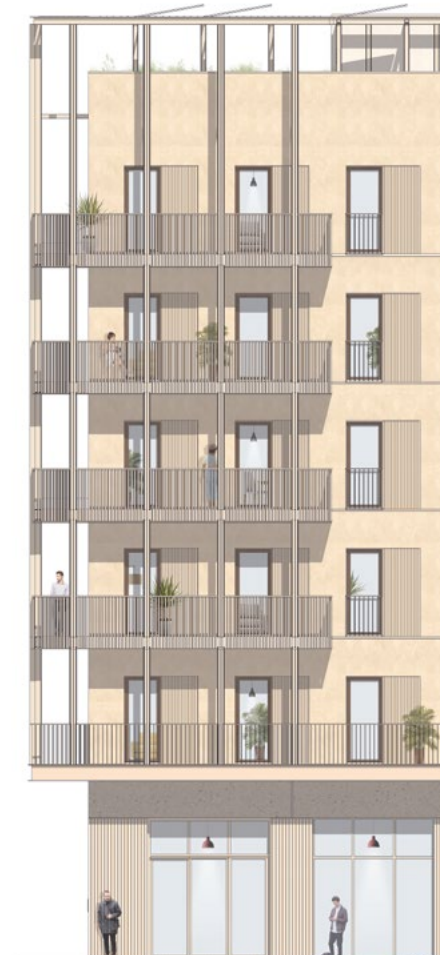
Focus on E2B3 timber structure building on a common precast concrete base
