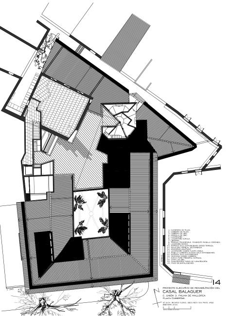
The roof around the patio used not to connect to the dome. The building's roof was previously an unstable and emergency construction, with a geometry that failed to channel the water to the outer perimeter, leaving it trapped at different points and thus damaging the palace's interior.
