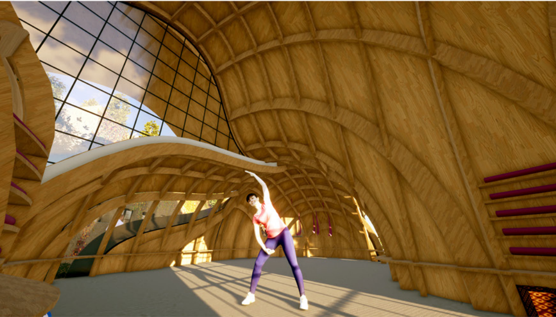
Photo 01 The interior space of the new Yoga Shala is governed by the Structural Beam Contours that form the supporting structure of the building. The wood ceiling enhances the warmth of the space.
