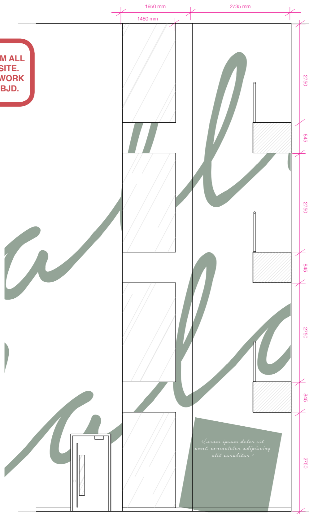
VOID AREA ELEVATION: GRAPHIC DECAL PATTERN APPLIED DIRECTLY TO THE WALL SURFACES THROUGHOUT THE ENTIRE VOID AREA WRAPPING IN PARTS TO FLOOR. COLOUR TO MATCH PANTONE 5635 C NB: ELEVATION NOT TO SCALE
