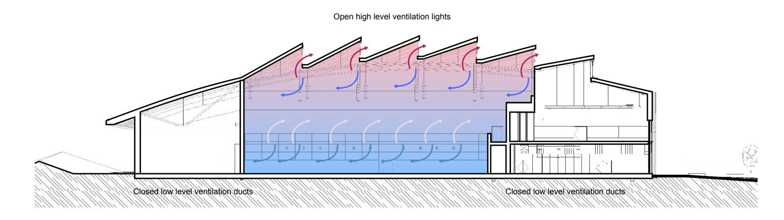
Closed low level ventilation ducts
