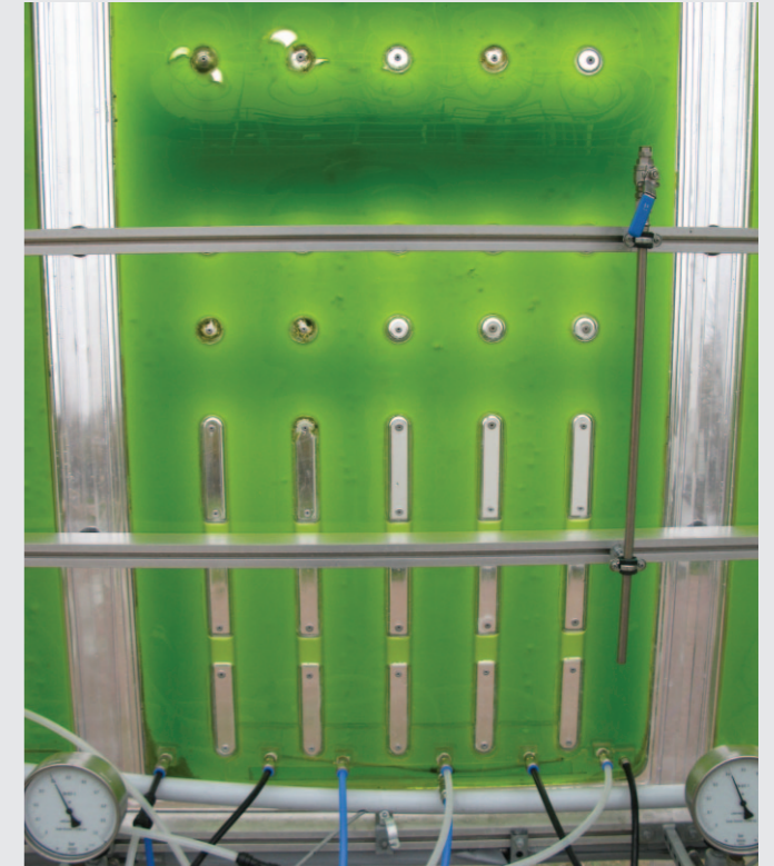
Backside of the flat panel PBR on an open field test site, where this technology was tested prior to this project
