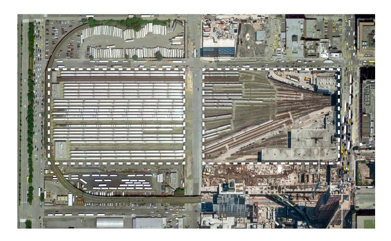
To build the first half of Hudson Yards, a "platform" was constructed over the Eastern Rail Yard of the Long Island Rail Road. A similar structure will be built over the Western Rail Yard. When completed, the two platforms will support approximately three quarters of the 28-acre primary development. The foundations of the buildings that sit on the platform extend through and rise above it.
