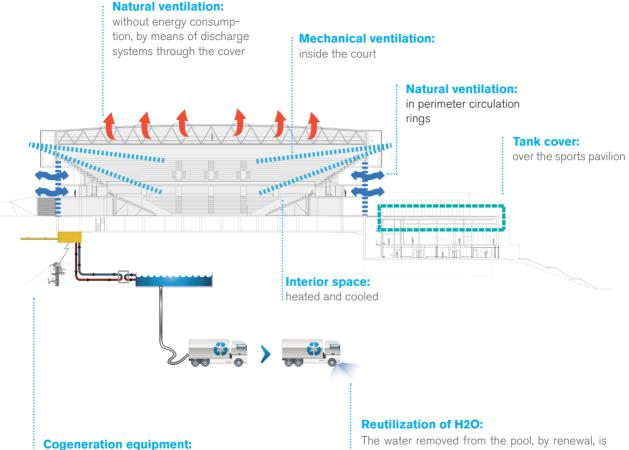
A cogeneration system produces electricity from natural gas and allows the obtainment of heat for the pool without producing additional costs
