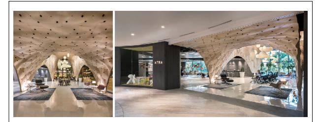
Compared with the Version 01 grid shell, this pioneering technique of tailoring plywood allows us to form a larger surface with drastically much lower number of modules: in this instance 280 panels as compared to 4,000 panels in Version 01. The installation of the Fabricwood panel is also comparatively much simpler and can be accomplished by unskilled labour.
