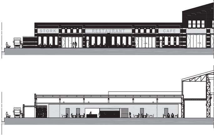
All facilities are placed behind one long continuous wall that doesn't reach the facades or the roof of the building. The large open industrial space is thus left intact; the new elements are treated as furniture-like additions. This wall contains several openings with one of them the open kitchen where all the cooking and preparation by the chefs is shown.
