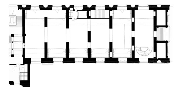
Modular showcases are installed between each buttress such that the layout can be changed on demand. Each showcase is connected to a technical support network along **two parallel paths which delimit the display zone and the public zone.**
