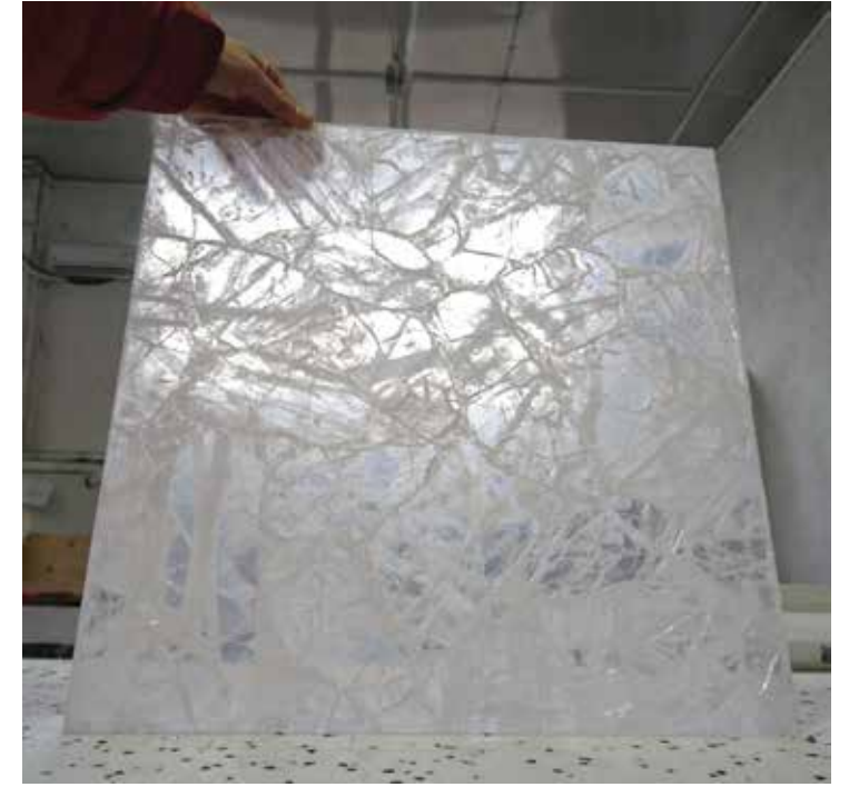
quartz crystal with two identical faces, both polished, 9 mm/0.35in thickness
