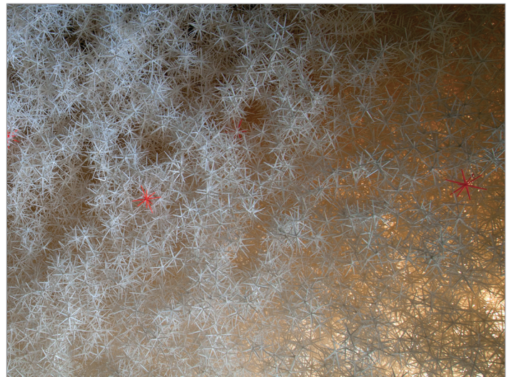
Image 2: The aggregate structures are self-supporting and require no further binding agent. The construction process can be either low-tech manually or high-tech digitally controlled. Variances in density of the granulate allow for the variation of material properties, such as thermal insulation or luminance effects. The designed aggregate thus allows for functional grading of architectural performance criteria within one and the same material system.
