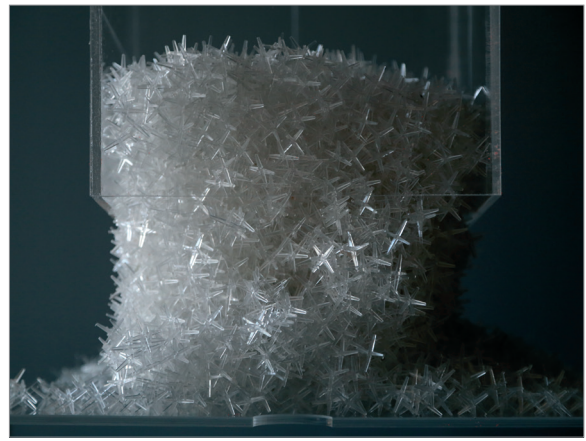
Image 4: Flow and stabilization test of designed granulate.
