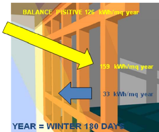
Figure n. 1 The amount of solar energy that enters through a window vertically oriented to the South, with high quality glass, is greater than that which is dispersed in the same period. In order to keep the heating the heat you need a good quality of heat insulation.
