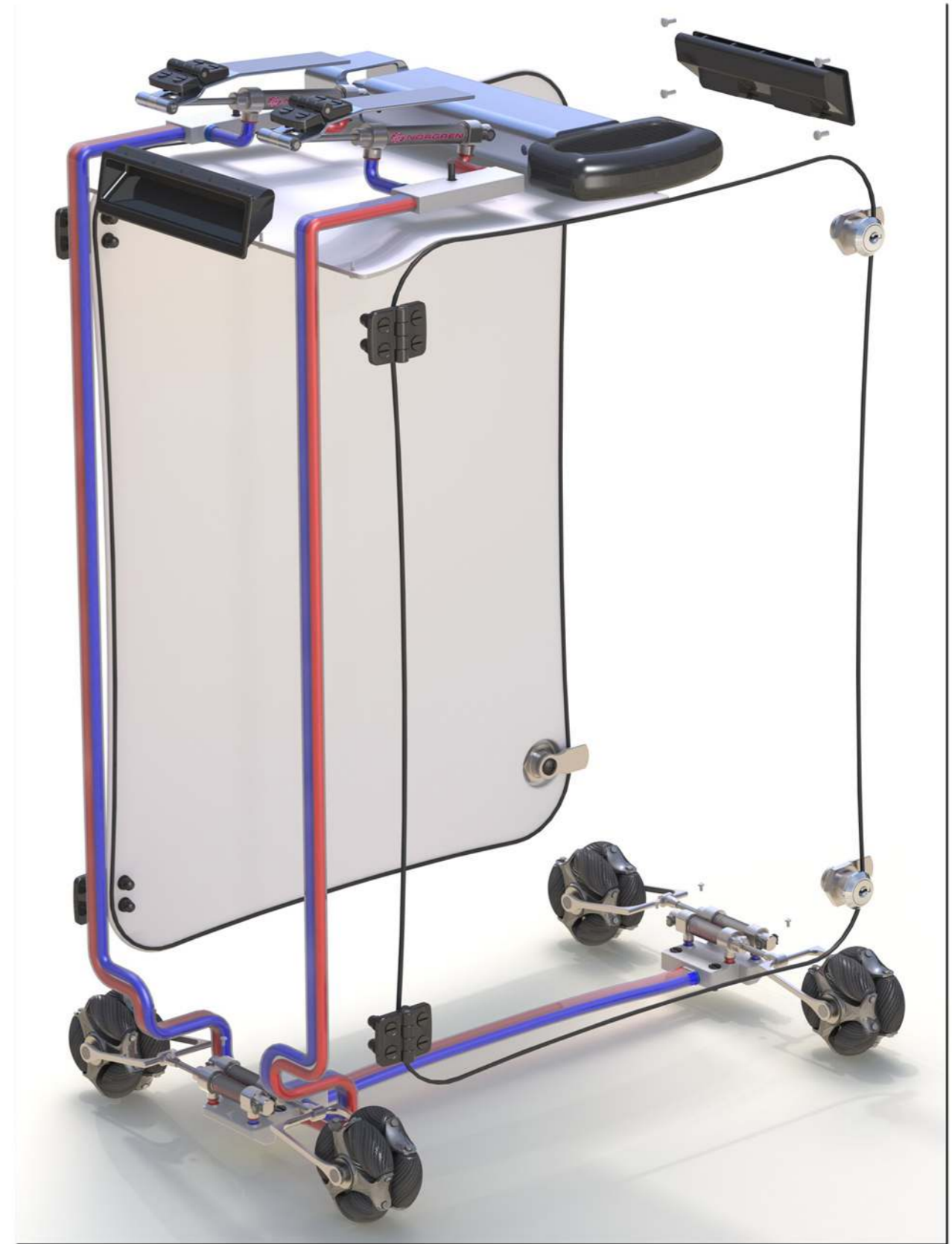
A complete overview of all the hydraulic components of the Samsonite suitcase. The cylinders are double action. This is being shown by the red and blue colours.
