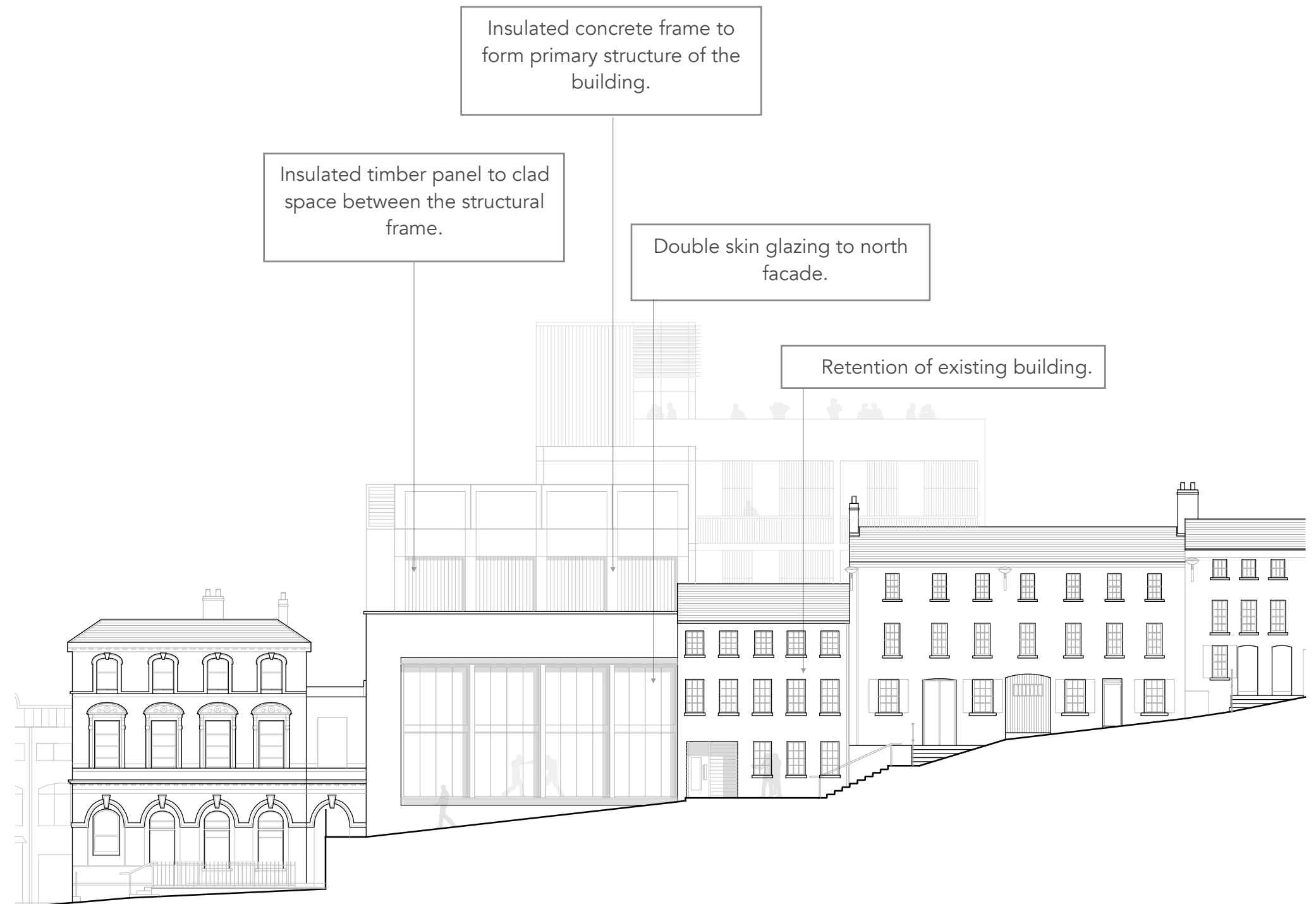
Fig. 3: NIBA North Elevation to Market Street / Scale 1:200
